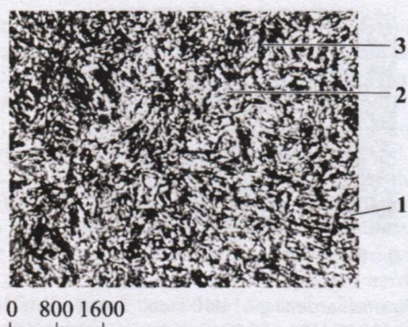
Fig. 9. Plasma hardening of U10 steel with local cooling. Hardening temperature 900 °C. M_s=+180 °C; M_f=-80 °C. Residual austenite (1) and secondary cementite (2) are present in the structure. The main structure is martensite (3) HRC 62–64. Magnification \times 400
