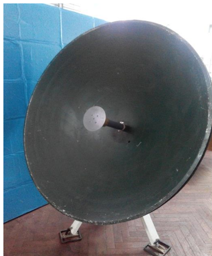
Fig.2 two-mirror antenna with an elliptical small mirror (ADE)
