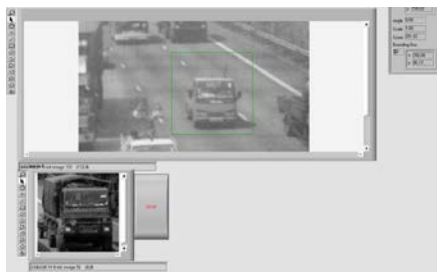
Fig. 40.49 – The result of the cars detection on the road (video stream)
