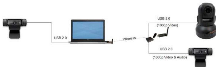
Fig. 40.8 – Using the USB web camera with/ without Wireless Extender
