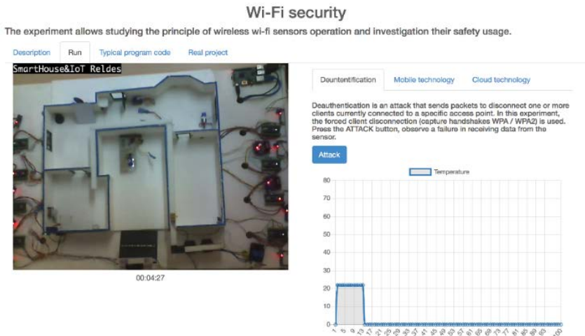
Fig. 38.11 – Experiment Wi-Fi security web-page
