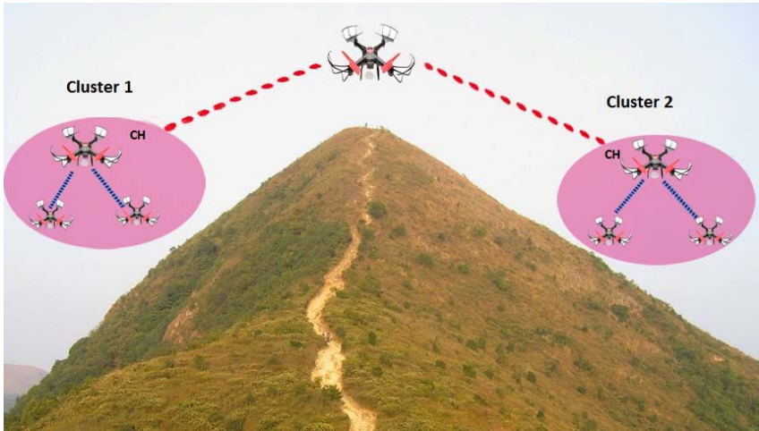
Fig. 43.14 – Multilevel Hierarchical Routing
