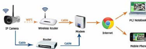
Fig. 40.10 – Example of IP camera usage
