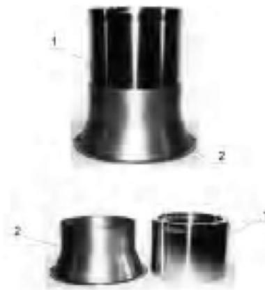
Fig. 54.4 – Fragments of the shaft of the compressor before and after treatment in the fluidized abrasive (1 - after turning; 2-after PSA)
