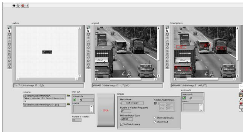
Fig. 40.47 – Result of cars detection on the road (images)
