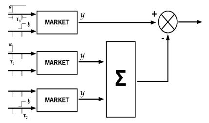
Figure 1 – Structural diagram of the procedure for identifying the second-order transition function for different inputs.
