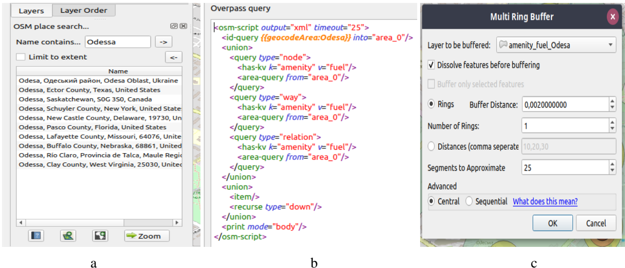
Fig. 3. Results of QGIS plugins settings for visualization of the filling station network as potentially hazardous objects: a – OSM Place Search plugin dialog box; b – OpenStreetMap server request script text; c – Multi Ring Buffer plugin dialog box Source: compiled by the author
