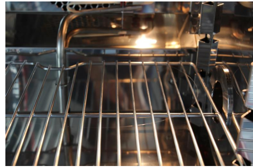
Fig. 7. Bragg's grating placed in climate chamber
