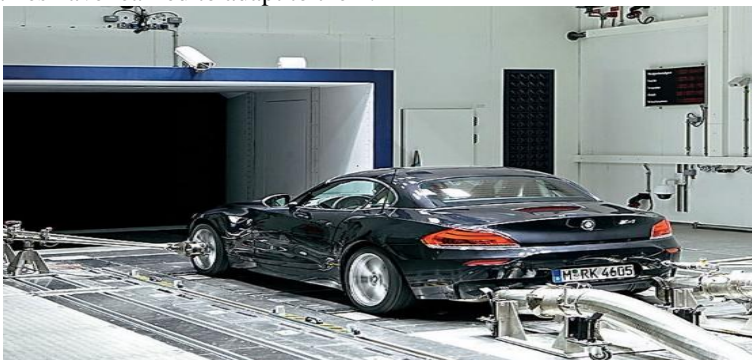
Fig.1. A running drum on which carbon footprint measurements are made
