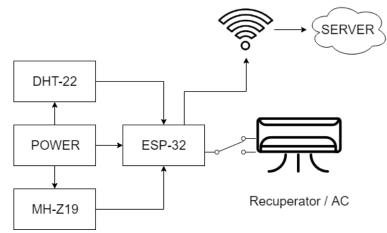
Fig. 3. Scheme of microclimate module
