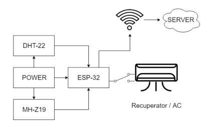
Fig. 4. Scheme of the microclimatic module
