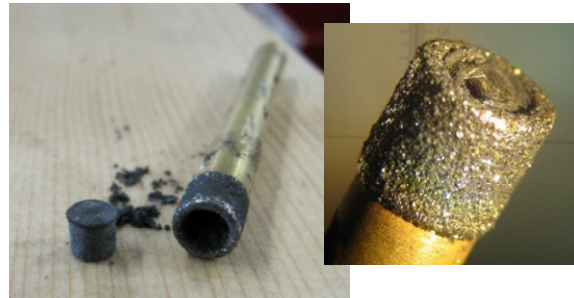
Fig. 7. The photos of core blocking
