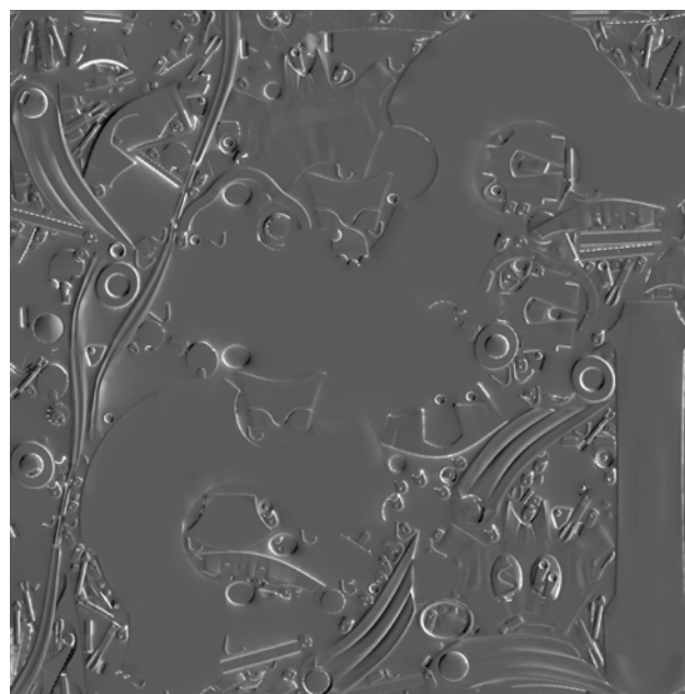
Fig. 4. Example of one of the four normal maps, which were used in the lowpoly model of robot on the fig. 1.
